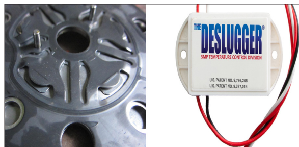
Figure 1: Slugging can damage reed valves. A "Deslugger" module will cycle the compressor rapidly on start up. Rapid cycling on start up allows the safe pump-out of any liquid refrigerant or oil which has accumulated after sitting for a specific amount of time.
