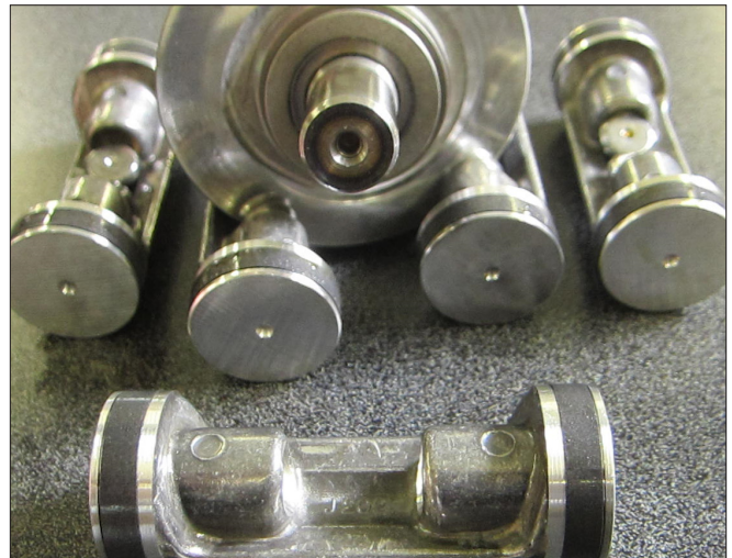
Figure 7: A swash plate allows for “fixed-displacement”, opposing cylinder operation.
