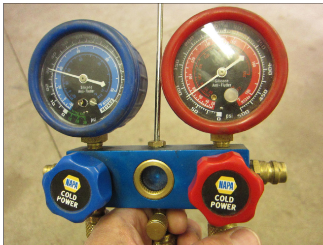
Figure 14: DO NOT get fooled with these readings on a variable displacement system. These readings represent a low refrigerant charge.
