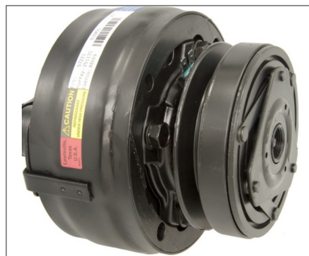
Figure 3: GM's R4 compressor would fail from reduced lubrication due to leaks causing a low refrigerant charge.
