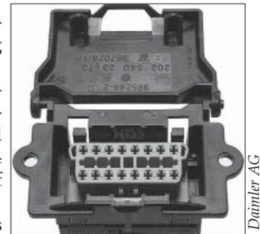
Figure 2: The common J1962 underdash VCI is archaic. It's 30+ years old, insecure and is limited to one user at a time
